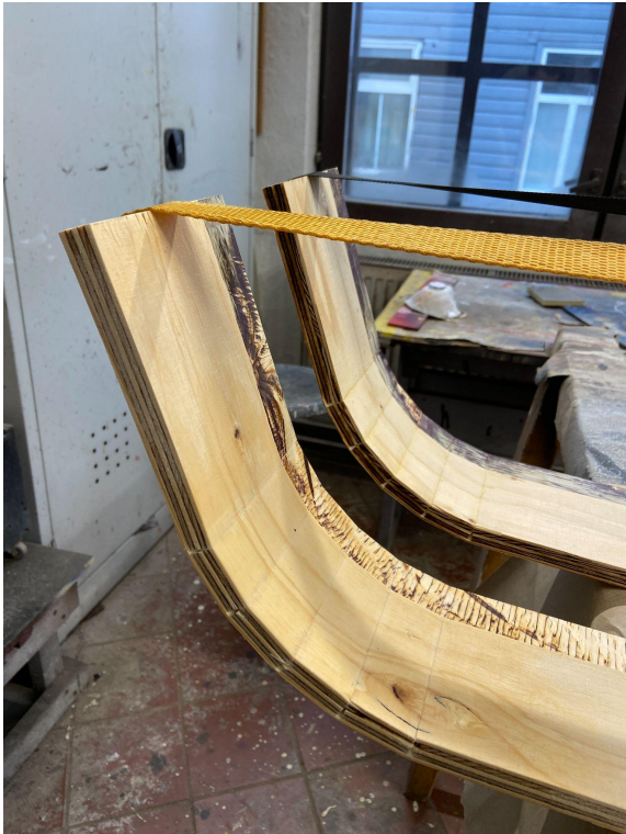
Foto 32. Kerf Cut meetodi abil detailide painutamine
