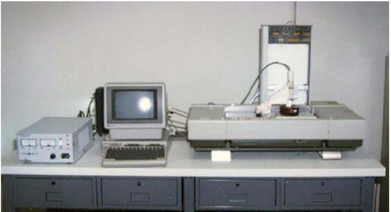
Foto 1. SLA-1 3D printer, mille valmistas Charles Hull (Gregurić, 2018)
