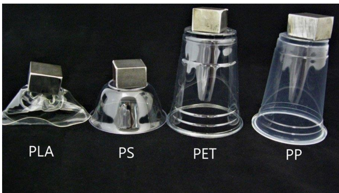
Figure 5 - Deflection under 0.3lb at 150°F
